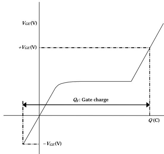
Fig. 7-1 Gate charge characteristics (Dynamic input characteristics).
