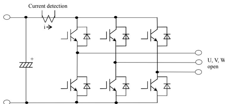
Insufficient dead time makes short circuit current much larger than  $dv/dt$  current.
